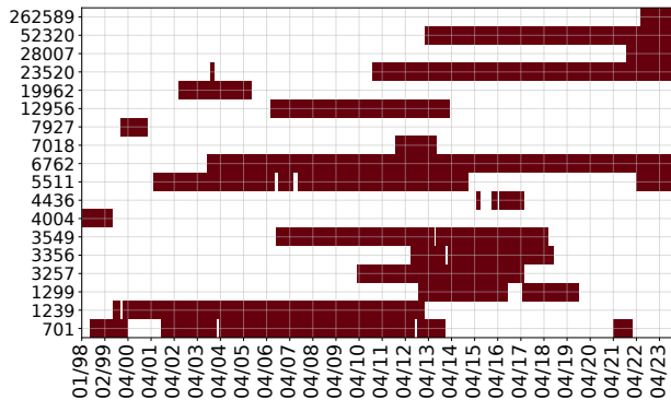
Figure 9: Changes over time in CANTV's upstream connectivity. Since 2013, excluding Columbus Networks (AS23520), all US-registered providers have ceased their services to CANTV, including Verizon (AS701), Sprint (AS1239), and AT&T (AS7018), GTT (AS3257 and 4436) in 2017, and Level3 (AS3356 and AS3459).
