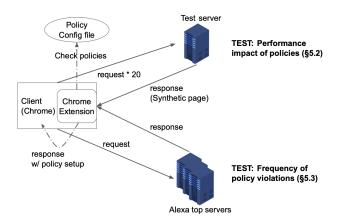
Figure 1: System diagram for the performance tests
