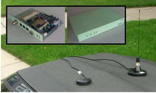
Figure 1. GPS and radio antennas installed on the roof of a vehicle. The car's windshield is visible in the lower left-hand corner of the image. The inset shows the internal hardware and exterior of the Soekris machine.
