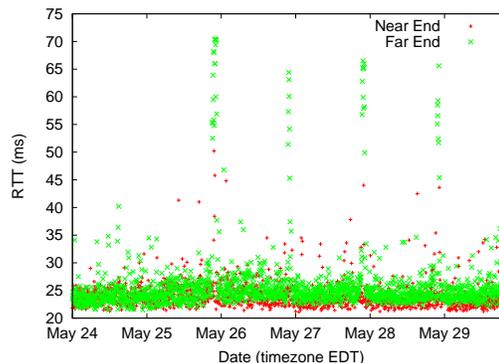
**Figure 3: An interdomain link between network C and D, measured from a VP within network C, in May 2015. TSP probes show moderate congestion on 4 days in 2015 for 1-2 hours during peak times in the local time zone of the VP.**
