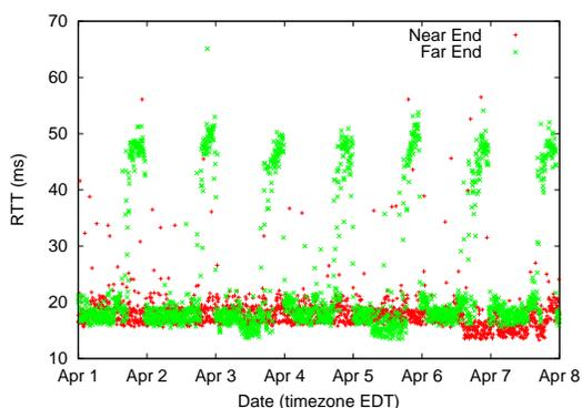
**Figure 2: Congestion on an interdomain link between network A and B, measured from a VP within network A, in April 2015. TSP probes show evidence of congestion for approximately 4-5 hours during peak times in the local time zone of the VP.**
