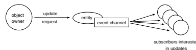
Figure 18: Achieving proactivity: when the owner of an object updates any of the object's attributes, notifications are sent to all interested clients.
