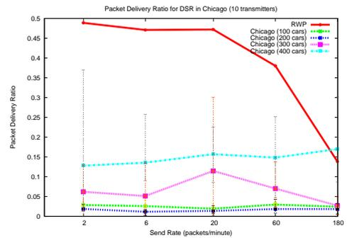
Figure 9: Comparison of DSR packet delivery ratio between mobility in downtown Chicago and the random waypoint model using 50 radio-equipped nodes and varying send rates.
