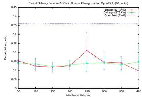
Figure 6: Comparison of AODV packet delivery ratio between mobility in downtown Chicago, Boston and the random waypoint model using 50 radio-equipped nodes.
